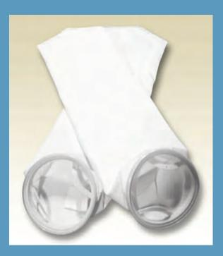
Needle Felt Filter Bags are the most economical disposable filter material available. They provide depth filtration and surfaces free of fiber migration while utilizing hot melt seamless welding technology to ensure effective filtration without filter bypass.
