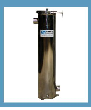
FSC1 bag filter housings are suitable for use in a wide variety of applications. V-Clamp lids allow for quick and easy bag change-outs, and floor mounting tabs provide the smallest possible footprint. FSC1 filter vessels fit industry standard size #2 bags. 304 stainless steel housings are stock items, 316L stainless steel is also available. 2" and 3" threaded connections are standard.
