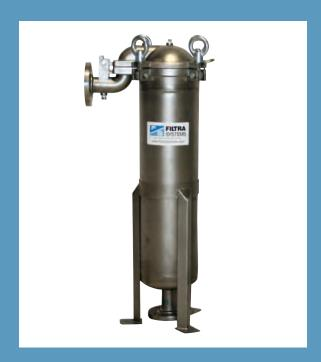
FSCT bag filter housings are used in more demanding applications. The gooseneck inlet configuration allows for laminar flow throughout the vessel. Vessel lids seal directly onto the bag, to prevent fluid bypass and minimize operator exposure to process liquid. ASME options are available. FSCT vessels fit industry standard size #2 bags. Carbon steel and 304 stainless steel housings are stock items, 316L stainless steel is also available. 2" ANSI flanged connections are standard.
