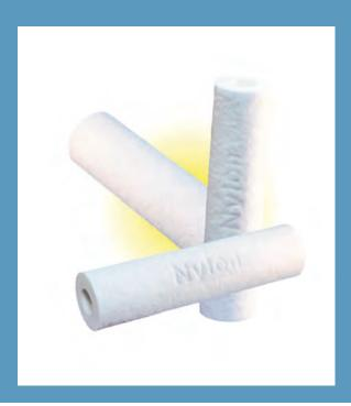
Super-Nylon filter cartridges are typically used to filter solvents, hydrocarbons, and in other applications in which polypropylene cannot be used. They are made without the use of binders or other adhesives, and a high void volume results in low differential pressure and a high dirt holding capacity.
