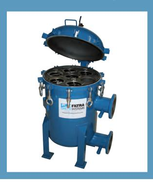
Multi-Bag Filter vessels with swing bolt lids allow for high liquid flow rates. A large variety of multi-bag vessels are available, with 3-12 bag vessels kept in stock. Flow rates up to 1200 gpm. FSSB vessels fit industry standard size #2 bags. Carbon steel and 304 stainless steel housings are stock items, 316L stainless steel is also available. 3"-8" ANSI flanged connections are standard.
