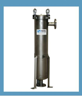
FSCS bag filter housings are suitable for use in high pressure applications. Swing bolt lids ensure that vessels are safe to use at pressures up to 150 psi, and mounting legs allow for a variety of possible vessel positions. FSCS filter vessels fit industry standard size #2 bags. Side outlet and bottom outlet housing configurations are available. Carbon steel and 304 stainless steel housings are stock items, 316L stainless steel is also available. 2" and 3" ANSI flanged connections are standard.
