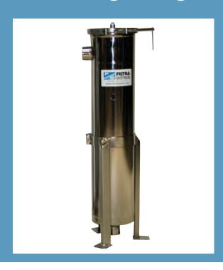
FSC2 bag filter housings are suitable for use in a wide variety of applications. V-Clamp lids allow for quick and easy bag change-outs, and mounting legs allow for a variety of possible vessel positions. FSC2 filter vessels fit industry standard size #2 bags. 304 stainless steel housings are stock items, 316L stainless steel is also available. 2" and 3" threaded connections are standard.
