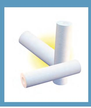
Super-Pure filter cartridges are typically used to filter process water, medium to low viscosity fluids, and as a prefilter for RO membranes. They contain an inner layer consisting of fine fibers, and a coarse-fibered outer layer for a high contaminant holding capacity.
