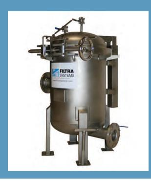
Multi-Bag Filter vessels with quick-change lids allow high liquid flow rates, with minimum downtime for bag change-outs. Individual units are available that can process flow rates up to 2300 gpm. FSQC vessels fit industry standard size #2 bags. Carbon steel, 304 stainless steel, and 316L stainless steel housings are available. 3"-10" ANSI flanged connections are available.
