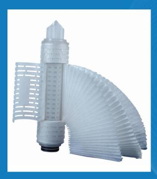
Poly-Ray filter cartridges are used when absolute filters are needed. These sanitary cartridge filters are effective to 0.2 micron absolute (99.9% efficient). They contain pleated sheets of melt-blown media for maximum removal efficiency.
