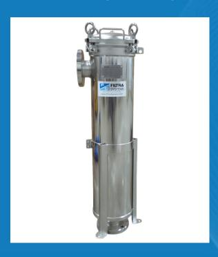
FSCS bag filter housings are perfect for use in high pressure applications. Swing bolt lids ensure that vessels are safe to use at pressures up to 150 psi. The mounting legs allow for a variety of possible vessel positions. FSCS filter vessels fit industry standard size #2 bags. Side outlet and bottom outlet housing configurations are available. 304 stainless is our standard build, but 316 stainless and carbon steel can be custom ordered. 2" and 3" ANSI flanged connections are standard.
