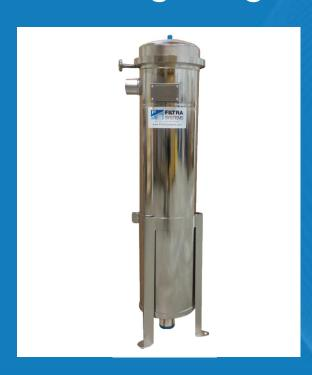
FSC2 bag filter housings are suitable for use in a wide variety of applications. V-Clamp lids allow for quick and easy bag change-outs, and mounting legs allow for a variety of possible vessel positions. FSC2 filter vessels fit industry standard size #2 bags. 304 stainless steel housings are stock items, 316 stainless steel is also available for custom order. 2" and 3" threaded connections are standard.
